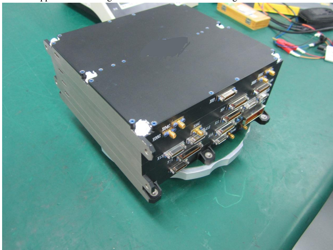
Fig.1 Micro-nano Satellite Integrated Electronics
